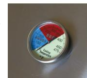
Thermometer located on canopy indicates the best zones for warming, smoking, and grilling.
